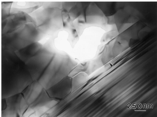
Fig. 7. TEM of microcrack (arrowed) at the interface between SiC platelets and mullite derived from kaolin/ \alpha -alumina hot pressed 1.5 h at 1600°C with 15 MPa pressure.
